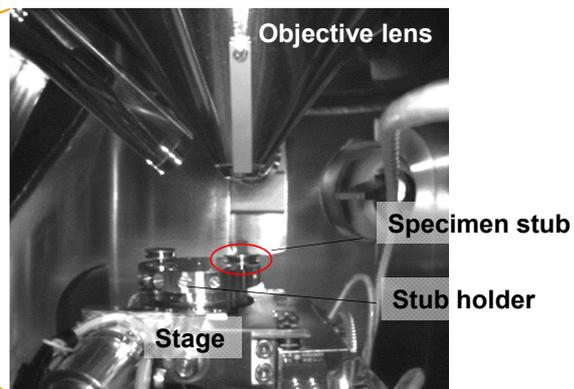
Specimen stage (x, y, z, r, tilt)
